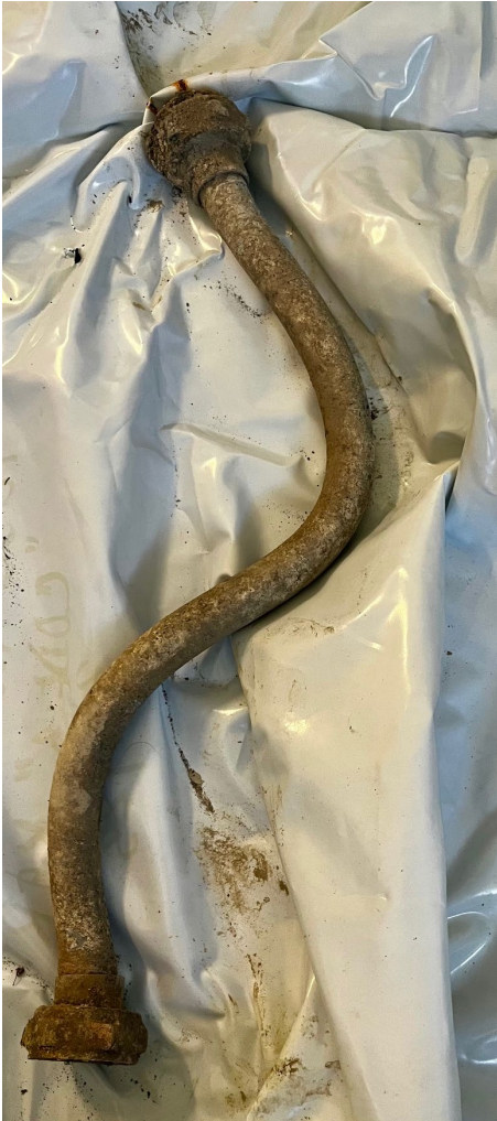
Lead gooseneck removed from Asbury St in San Jose 2023
