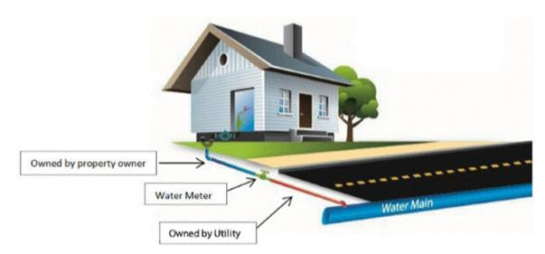
NOTE: Under SB 427 and previous California regulations, the sections of the service line titled "Owned by Utility" and the "Water Meter" are included in California's definition of a "service line." The EPA's new LCRR expands the definition of "service line" to also include "Owned by property owner" such that the entire line, regardless of ownership, is required to be included in a water system's inventory.
