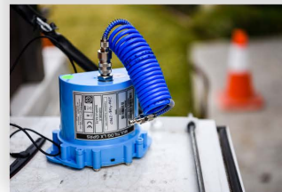
Newly installed tank mixing systems (top) and remote pressure monitors will provide continuous monitoring of SJWC's system and water quality
